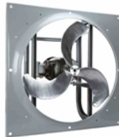
16" EXPLOSION PROOF LOW PRESSURE FAN - 2950 CFM - 1/4 HP - 115V - C1 GROUP D & C2 GROUPS F & G
