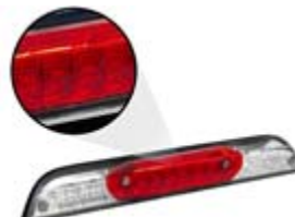
LED Lights have "squares" behind the lens and no replaceable bulb.
