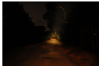
This image shows the HML-5M illuminating the same dark road as above, easily reaching distances of up to 500'
