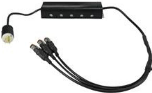
**The Larson Electronics DCP-25-3XDP Waterproof Power Supply converts commonly used 120 - 240VAC electrical current to 12VDC @25 Amps. This converter includes a typical straight blade plug on the input end and three 2-prong Deutsch connectors on the output end. This unit takes voltages within the 100-277VAC range and reduces it to 12/24 VDC, allowing users to use standard AC power to operate equipment like our LED light bars and HID Golights that require low voltage DC current.**
