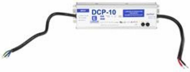
The Larson Electronics DCP-10-24V Waterproof Power Supply converts commonly used 100-277VAC electrical current to 24VDC @10 Amps. This converter is designed to be hardwired into building, boat or vehicle electrical supplies and takes voltages within the 100-305VAC range and reduces it to 24VDC, allowing users to use standard AC power to operate equipment like our LED light bars and HID Golights that require 12 Volts DC.
