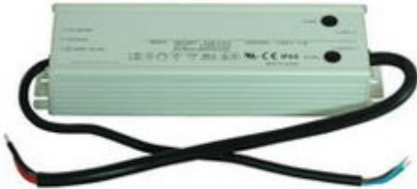
**The Larson Electronics DCP-6-24V Power Supply converts commonly used 100 - 277VAC electrical current to 24VDC @6.25 Amps. This converter is designed to be hardwired into home, boat or vehicle electrical supplies where the voltage is typically within the 100-277VAC range and reduces it to 24VDC, allowing users to use standard AC power to operate equipment like our LED light bars and HID Golights that require 24 Volts DC.**
