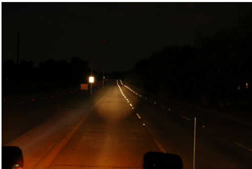
Halogen Golight illuminating a stretch of road about 5000 feet in length. Beam loses intensity after 750'.
