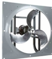
12" EXPLOSION PROOF LOW PRESSURE FAN - 970 CFM - 1/4 HP - 115/230V - C1 GROUP D & C2 GROUPS F & G
