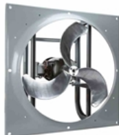
12" EXPLOSION PROOF LOW PRESSURE FAN - 970 CFM - 1/4 HP - 115/230V - C1 GROUP D & C2 GROUPS F & G
