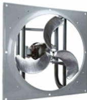
24" EXPLOSION PROOF FAN - 7820 CFM - 1 HP - 115-230V - CLASS 1 GROUP D & CLASS 2 GROUPS F & G RATED
