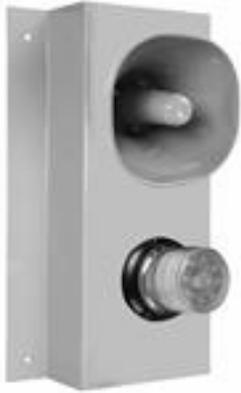
The SLEDB-CL1B-MS-PA-24V from Larson Electronics is an LED Motion Alarm System w/ Horn for industrial use. This 24V DC unit features a Class 1 LED strobe light and audible horn that can produce eight different tones to sound levels up to 110 dBA @ 10 feet. A pre-drilled aluminum base facilitates wall, ceiling or surface mounting applications.
