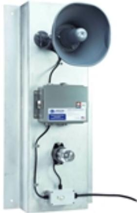
**The SLEDB-CL1B-MS-PA-12V from Larson Electronics is an LED Motion Alarm System w/ Horn for industrial use. This unit features a Class I LED strobe light and audible horn that can produce eight different tones to sound levels up to 110 dBA @ 10 feet. A pre-drilled aluminum base facilitates wall, ceiling or surface mounting applications.**
