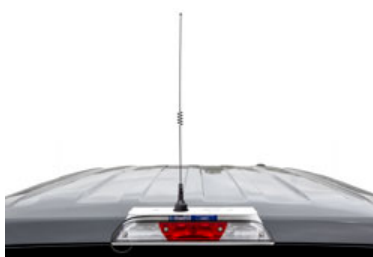
VMP-AM-FRPT-2017-LED Aluminum Plate For Mounting Permanent Mount Antennas
