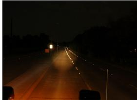
Halogen Golight illuminating a stretch of road about 5000 feet in length. Beam loses intensity after 750'.
