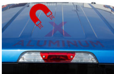
Aluminum Body is Not Magnetic
