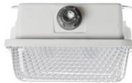
This Class 1 Division 2 rated fixture is constructed of non-corrosive materials including a polyester housing reinforced with glass fiber, a poured in gasket for reliable sealing and an impact resistant acrylic diffuser. Eight corrosion resistant plastic latches secure the lamp cover to the housing and provide a firm lock against the poured in seal to prevent drips and water intrusion.
