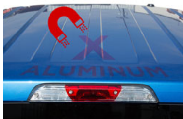
Aluminum Body is Not Magnetic
