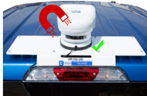
MMP-V2-FSD-2017 Steel Plate is Magnetic
