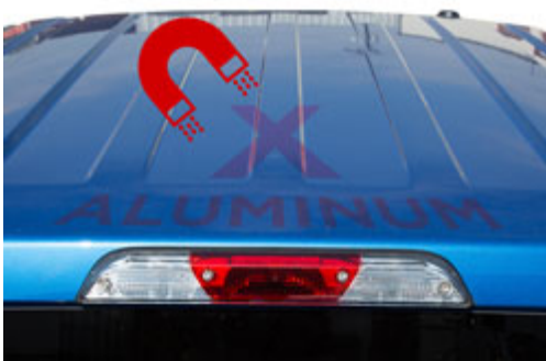
Aluminum Body is Not Magnetic
