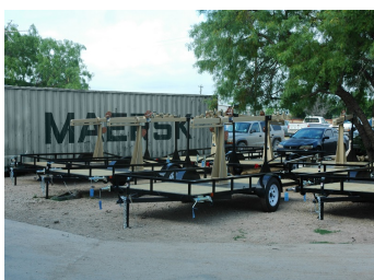
The LM-30-3S-ATM-TLR fitted with four HID-22-SL-REM 1000 Watt Metal Halide Light Fixtures
