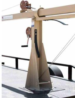
Manual 1,000 lb hand crank winch for elevating and folding over the light mast on the LM-30-3S-ATM-TLR.
