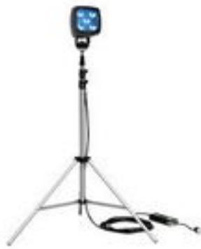
**The WAL-TP-LEDWL-25W-BLU-25-1227 from Larson Electronics is a Blue LED Spotlight with Aluminum Tripod Mount that produces 2250 lumens of high intensity blue LED light while drawing only 25 watts and offering operators a versatile and flexible lighting solution for a wide variety of tasks. This LED spotlight operates on 120-277V AC that is stepped down to 12V via inline transformer and is equipped with a choice of general area cord caps.**
