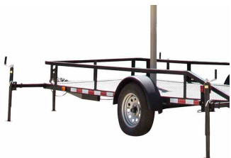
Retractable outriggers with 1,000 lb manual crank jacks and tail lights.
