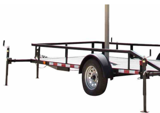
Retractable outriggers with 1,000 lb manual crank jacks and tail lights.
