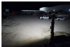
(4) 60 Watt LED Lamps Turned On Illuminating Wall 200ft. Away (20,000+sq.ft. area)
