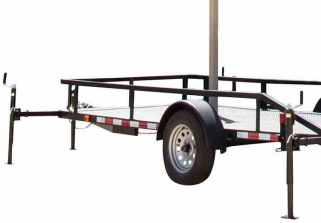
Retractable outriggers with 1,000 lb manual crank jacks
