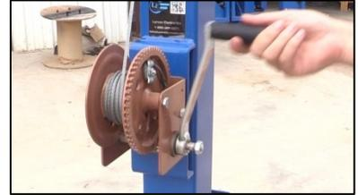
**WARNING:** Power cables can become pinched or tangled around light mast while lowering or rotating. Take caution in keeping cables clear.
