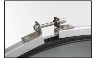
2. Carefully remove the outer ring, glass lens and rubber seal.
