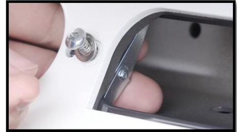
7. Once the mount is aligned, tighten the 2 toggle bolt screws with a Phillips screwdriver. Be careful not to over tighten these screws to prevent damage to the bolts and/or your truck. However, ensure that the screws used to compress the gasket are evenly tightened. Uniformly sealing the plate to the truck and firmly compressing all areas of the gasket.
