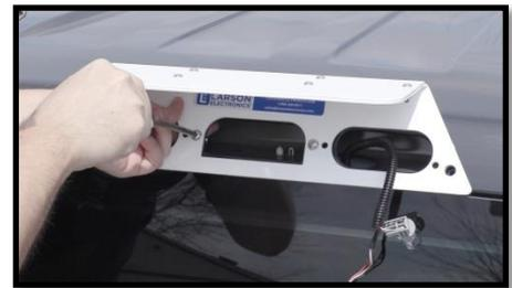
8. Reattach each light assembly to the brake light housing and twist to lock it in place. For taillights with a camera, reattach the wire harness.
