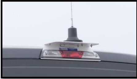
**Complete!** Your new mount is now installed! Check to ensure everything is secure and that your tail lights are working. Attach your device to the steel mounting plate via magnet (if applicable) or permanent mount to the aluminum plate. Run wires to your device.
