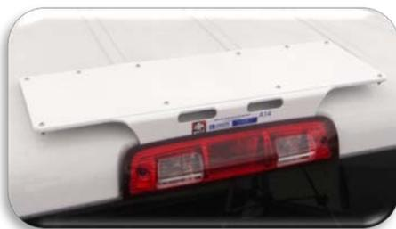
**Complete!** Your new mount is now installed! Check to ensure everything is secure and that your tail light is working. Attach your device to the steel mounting plate via magnet or permanent mount to the aluminum plate. Run wires to a power source. See page 3 for Routing Wire through Gasket.
