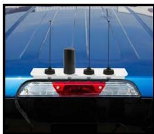
**Complete!** Your new mount is now installed! Check to ensure everything is secure and that your tail lights are working. Attach your device to the steel mounting plate via magnet (if applicable) or permanent mount to the aluminum plate. Run wires accordingly.
