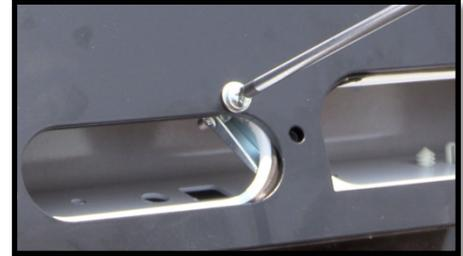
7. Position the mount so all the holes align properly and tighten the Phillips screws. Be careful not to over tighten these screws to prevent damage to the bolts and/or your truck. However, ensure that the screws used to compress the gasket are evenly tightened. Uniformly sealing the plate to the truck and firmly compressing all areas of the gasket.
