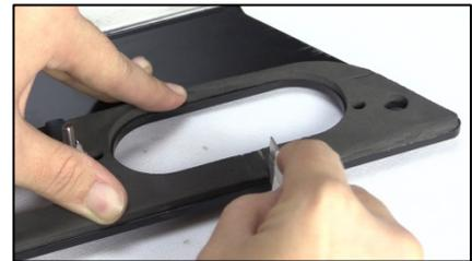
4. Test wire for fit. Cut any additional foam if necessary.
