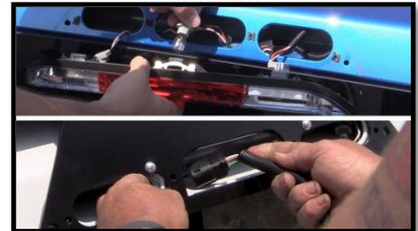
9. Place the brake light housing up against your truck and replace the 4 screws to hold it back in place.
