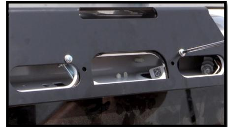
8. Reattach each light assembly to the brake light housing and twist each light to lock it in place. For taillights with a camera, reattach the brake light wire harness.
