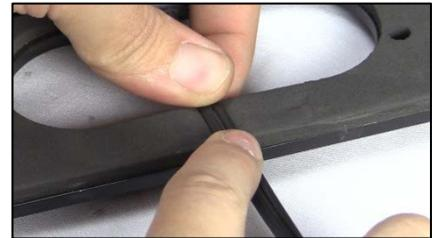
3. Cut gasket to size using indentation or marked area. Cut slightly smaller for a tighter fit and remove excess foam.
