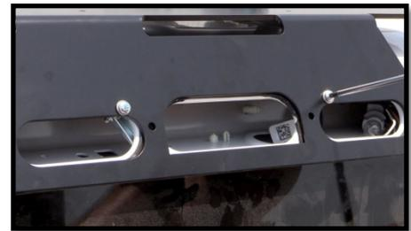
8. Reattach each light assembly to the brake light housing and twist each light to lock it in place. For taillights with a camera, reattach the brake light wire harness.
