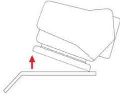
**Note:** When removing an attached magnetic device from the mounting plate, do not force the device off the front causing the mount to bend as this could cause strain to the mount and tail light. Instead, remove the magnetic device from the back of the mount, up and away from you.
