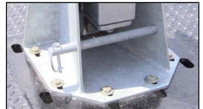
5. Replace the cable preventing the mast from extending during transport.
