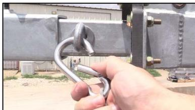
6. Replace the top retaining pin of the mast holder.
