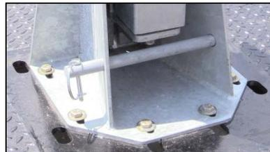
6. Use the upper hand winch for extending the mast. Turn this clockwise until it stops. You should hear a clicking noise from the hand winch indicating the proper direction. **Do not force the winch any further passed its stopping point!**
