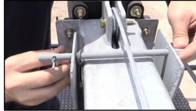
2. Unlatch the cable preventing the mast from extending during transport.
