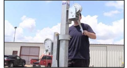
**WARNING:** Ensure the mast retaining pin is installed at the base of the mast before elevating!
