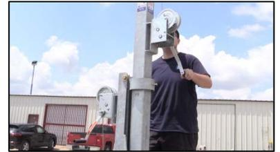
2. **Remove the retaining pin from the base of the mast and set aside.**
