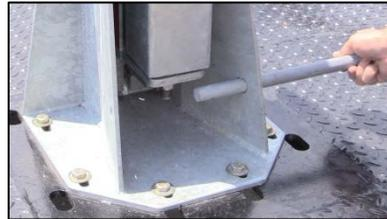
4. Use the lower hand winch to fold the mast upright. Turn this clockwise until there is enough tension keeping the mast in place. You should hear a clicking noise from the hand winch indicating the proper direction.
