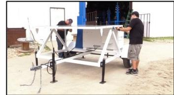
6. Lift the (4) jacks on each corner of the trailer by rotating the hand crank counter-clockwise. Pull the pin and rotate each jack 90°.
