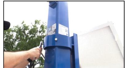
Note: Pay attention to any attached cords while rotating the unit to prevent tangles or strain around the light mast.
