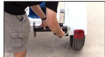
7. When the mast is fully lowered, powered off, and the (4) main jacks are raised, you are ready to attach a tow vehicle. Once tied to a tow vehicle, raise the tow jack and ensure all other outriggers are raised. Ensure the trailer hookup and safety chains are connected. Test trailer lights to ensure stop/tail/brake lights work before operating on public roadways.
