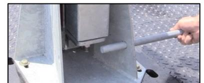
3. Use the lower hand winch to fold the mast down. Rotate the winch counter-clockwise until there is no more tension on the cable and the mast is set in its holder.
