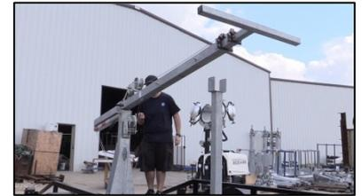
9. **Replace the pin removed in Step 3!** This retaining pin will prevent the mast from falling over should the winch cable fail.
