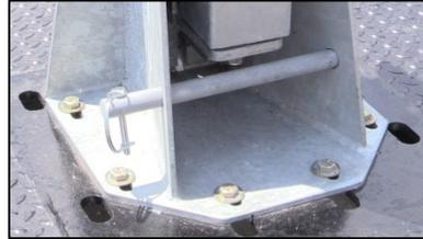
5. Replace the cable preventing the mast from extending during transport.
