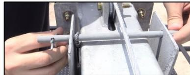
6. Unlatch the cable preventing the mast from extending during transport. (If applicable)
