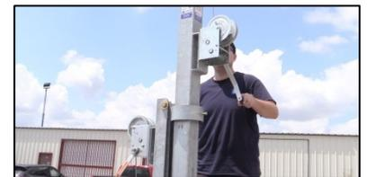
2. **Remove the retaining pin from the base of the mast and set aside.** This pin must be removed before folding the mast!
