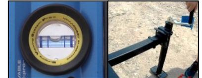
11. Use the upper hand winch for extending the mast. Turn winch clockwise until it stops. You should hear a clicking noise from the hand winch indicating the proper direction. **Do not force the winch any further passed its stopping point!**
