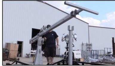
4. Replace the retaining pin on the base of the mast removed in **Step 2**.
