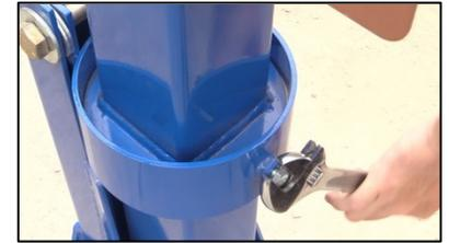
When using power cables, minimize full 360° rotation to prevent tangling cord around light mast. *Ensure cables are not in the way or tangled when lowering mast!*
