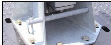
8. Use the lower hand winch to fold the mast upright. Turn this clockwise until there is enough tension keeping the mast in place. You should hear a clicking noise from the hand winch indicating the proper direction.
