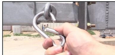
7. Remove the retaining pin from the base of the mast and set aside.
