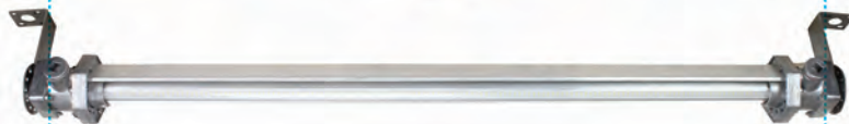
EXPLOSION PROOF LOW PROFILE LED LIGHT Class I, Division 2 Class II, Divisions 1 & 2 Dimensions: 50"L x 5"W x 3"H Voltage: Universal 100-277 VAC, 50/60Hz or 11-25V AC/DC Paint Spray Booth Approved 104 Watts - 13,520 Lumens Beam Angle: 100° Horizontal, 140° Vertical Part # EPL-48-100LED-SFC
